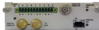
Rear panel includes electrical digital and analog video inputs, analog or AES audio inputs, electrical output and SFP transceiver cage
