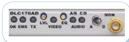
Front panel monitoring and status displays
