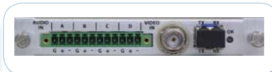
Real panel includes electrical video input, analog or AES audio inputs and SFP transceiver cage
